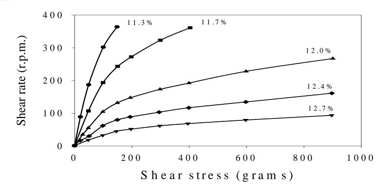
Dilatant flow of a series of suspensions of red iron oxide in an aqueous solution of sodium lignin sulfonate at 10% concentration at 30° C. The volume concentrations of solids are noted on the curves.
