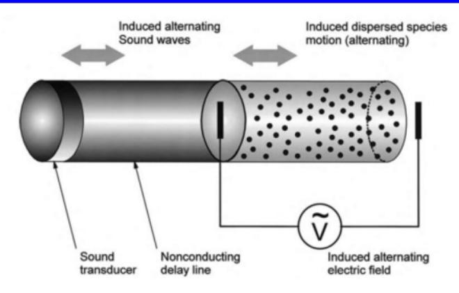
The ESA effect is measured by applying a field to the electrodes and listening for the sound in the transducer.
