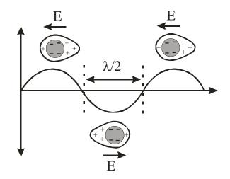
The technique uses an ultrasonic pressure wave to perturb the equilibrium double layer. This polarization generates an alternating electric field called the Colloid Vibration Potential:
