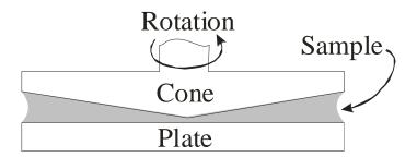
Consists of a flat plate and a cone with an apex angle of nearly 180°
