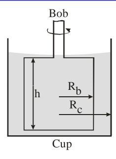
In modern Couette viscometers the bob is either driven with a known stress and the resulting angular velocity measured or it is driven at a known angular velocity and the required stress measured. The first provides viscosity as a function of shear stress, the latter provides viscosity as a function of shear rate.
