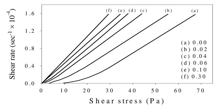
Rheograms of 20 w% deionized kaolin slurries at several levels of tetrasodium pyrophosphate\* addition. The figures on the curves indicate percent TSPP per weight of clay. An extrapolation of the linear region determines an apparent yield point.
